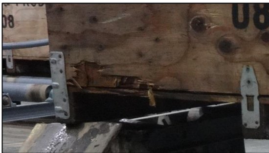
Whether plastic or wooden, bins should be inspected before each use to monitor for damage, such as scratches or cracks, that may harbor Listeria
