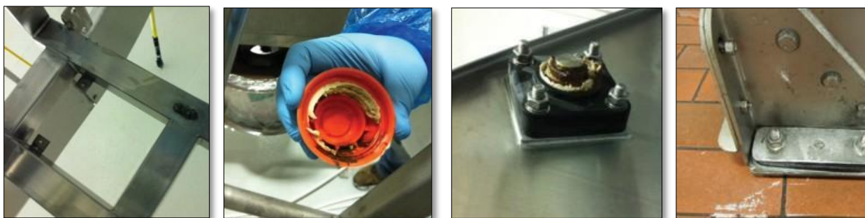
When sampling, consider hard to reach and rarely cleaned areas, particularly joints and attachment points.
