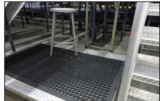
Anti-fatigue mats (and the floors beneath them) should be on a regular cleaning schedule to prevent bacterial harborage
