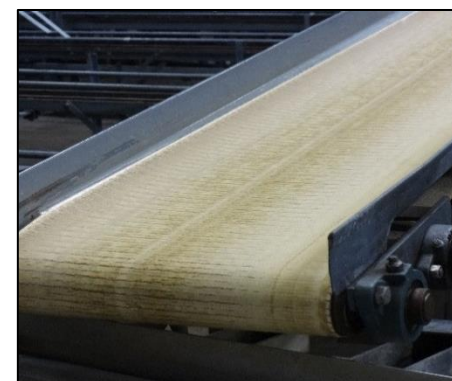
Old, cracked conveyor belts cannot be cleaned effectively and should be replaced
